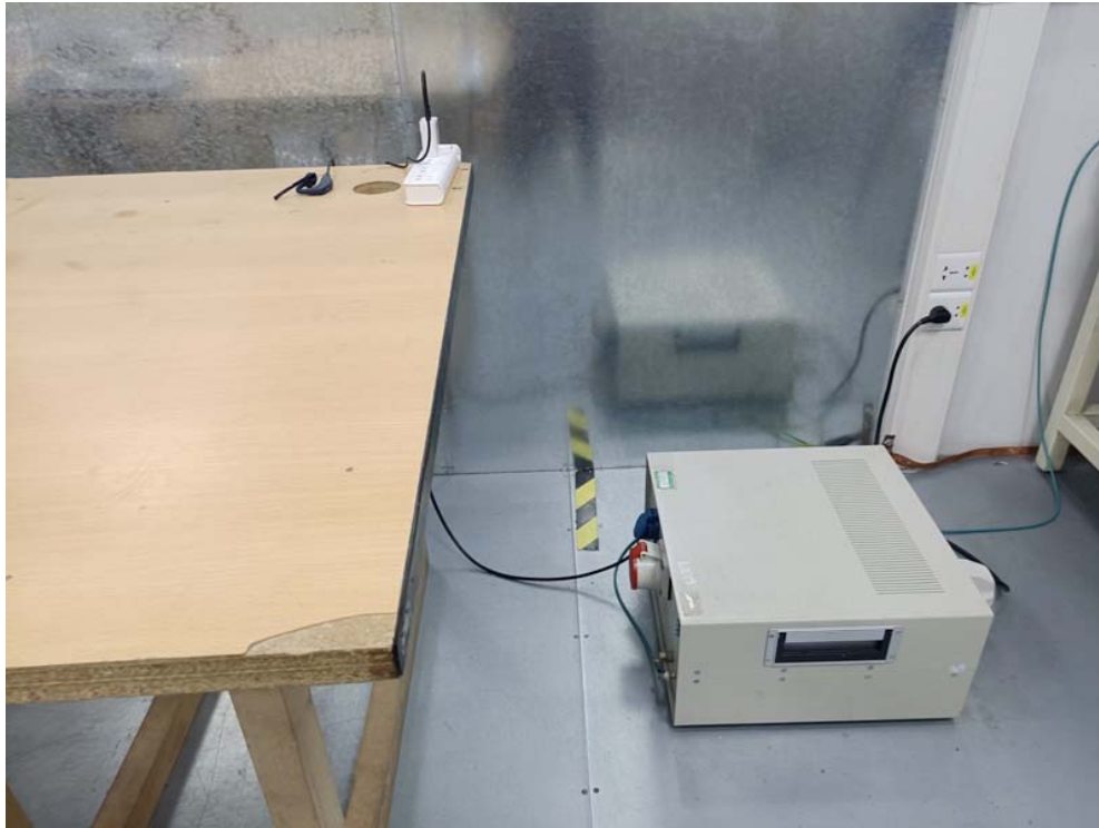
Conducted Emission Test Setup:
