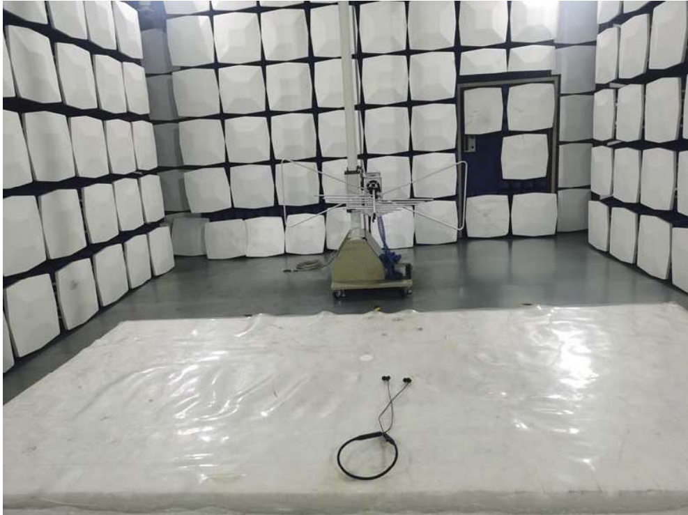
Radiated emission test view
