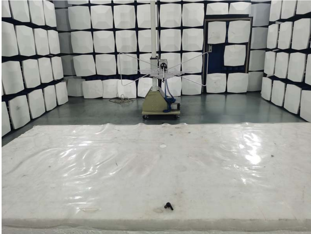
Radiated Emission Test Setup:
