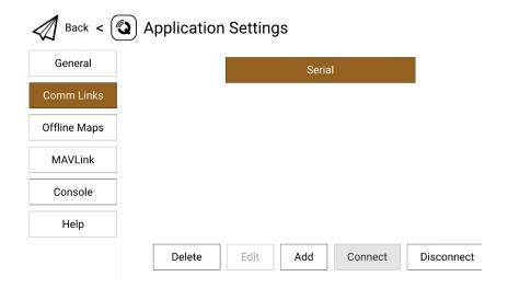
5. Touch the configured "Serial" connection and touch "Connect", USB COM (Serial) connection is finished.
