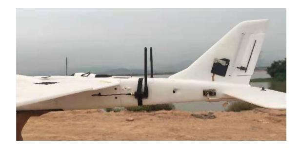
Antenna feeder wires should be placed away from devices with much current and heavy interference, such as ESC and motors.
