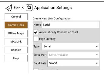
4. Name the connection as "Serial", set the type as "Serial" and the baud rate as "57600", then touch "OK" to return to the Comm Links page.
