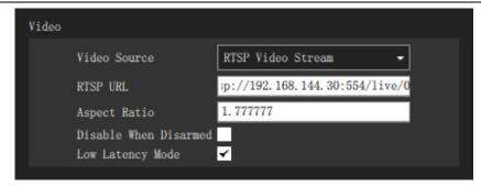
In "RTSP URL", input the RTSP address of the camera or HDMI converter connected with MK15 receiver, then you will see the image from the camera or HDMI converter.
