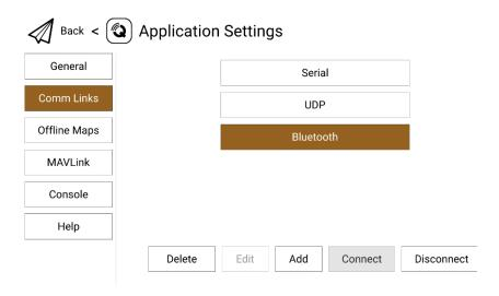
6. Touch the configured "Bluetooth" connection and touch "Connect", Bluetooth connection is finished.
