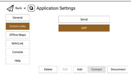
4. Touch the configured "UDP" connection and touch "Connect", UDP connection is finished.
