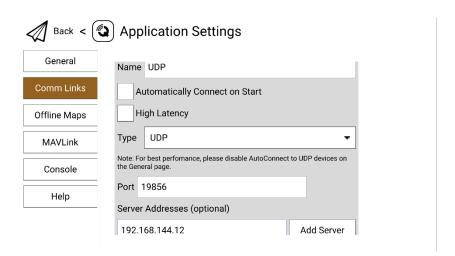
3. Name the connection as "UDP", set the type as "UDP", the port as "19856", the server address as "192.168.144.12" and "Add Server", then touch "OK" to return to the Comm Links page.
