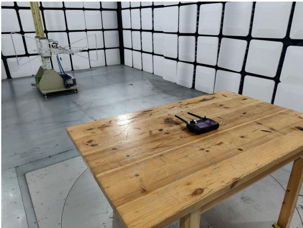
Photo of Radiation Emission Test
