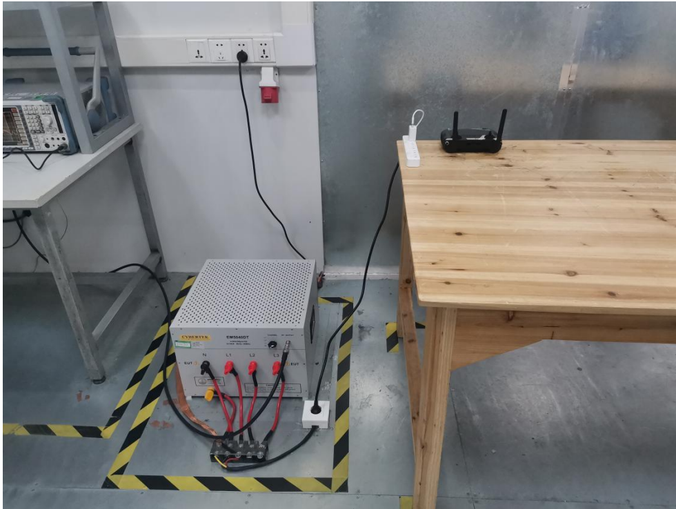
Photo of Power Line Conducted Emission Test
