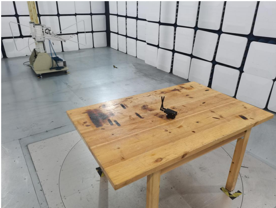
Photo of Radiation Emission Test
