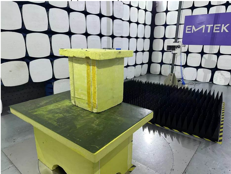
Spurious Emission Test Setup (Above 1GHz)
