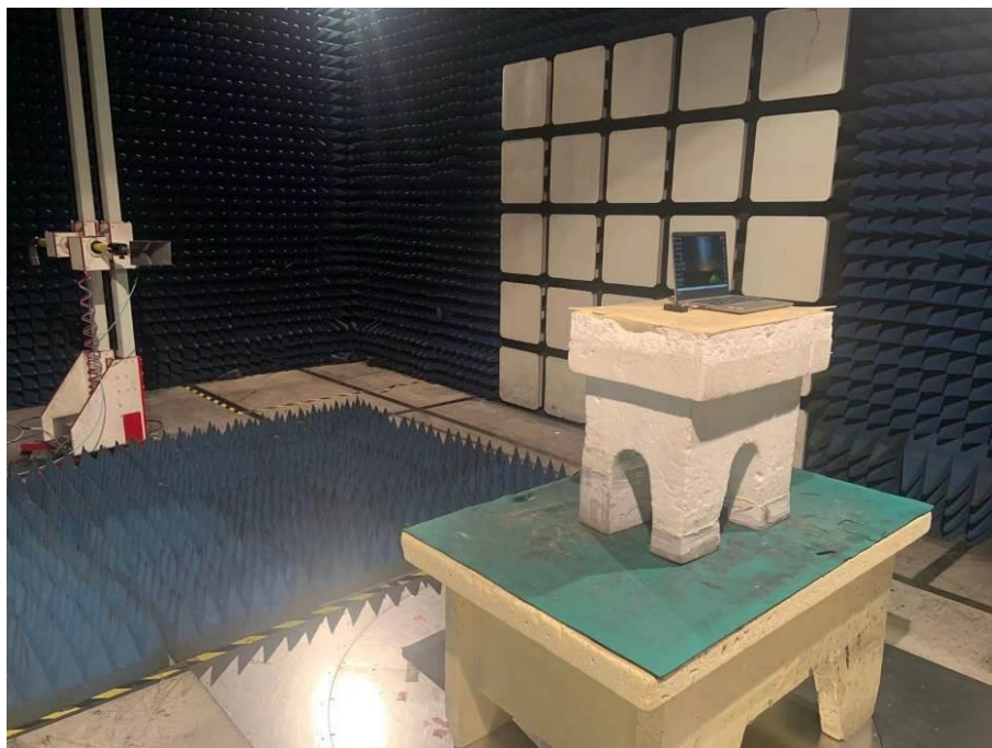
Spurious Emission Test Setup (Above 1GHz)
