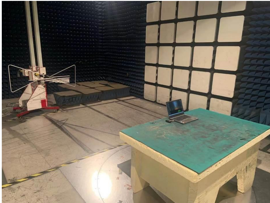
Spurious Emission Test Setup (Below 1GHz)
