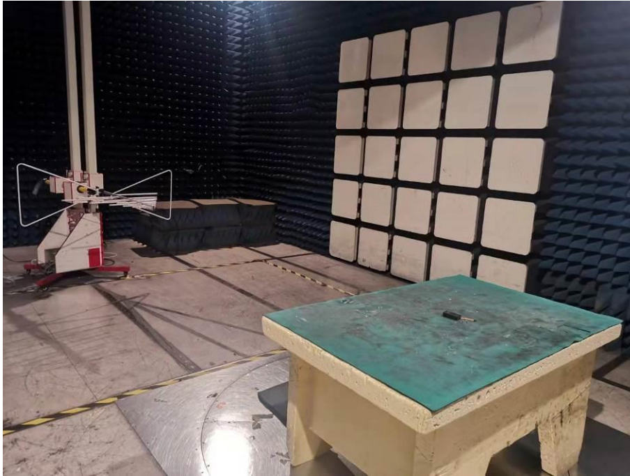
Spurious Emission Test Setup (Below 1GHz)
