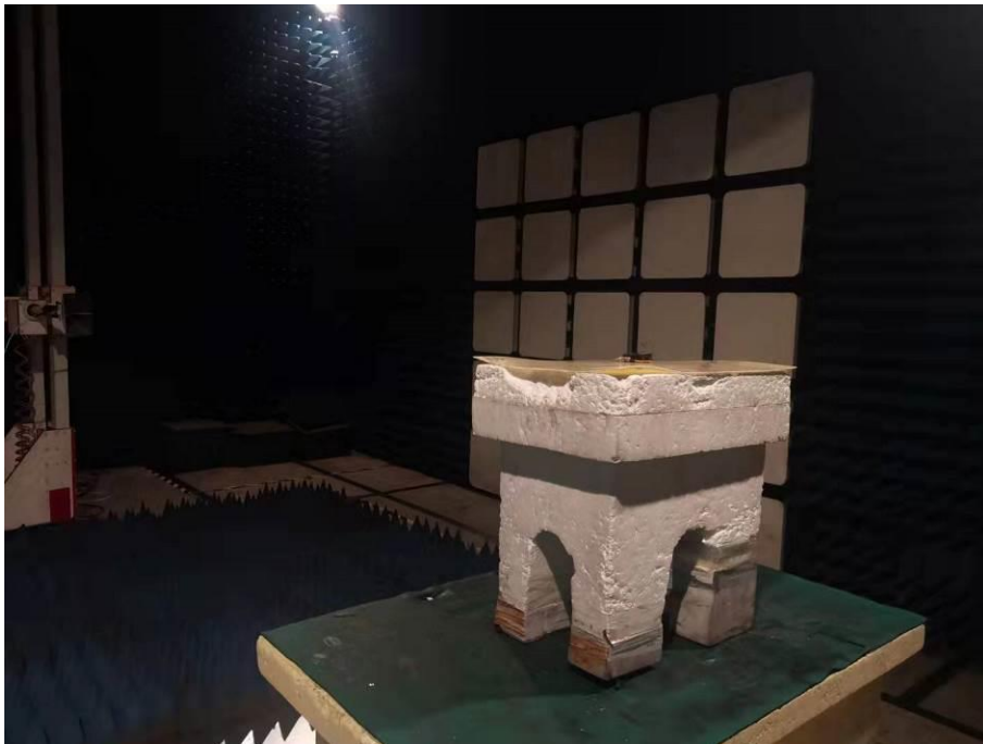
Spurious Emission Test Setup (Above 1GHz)
