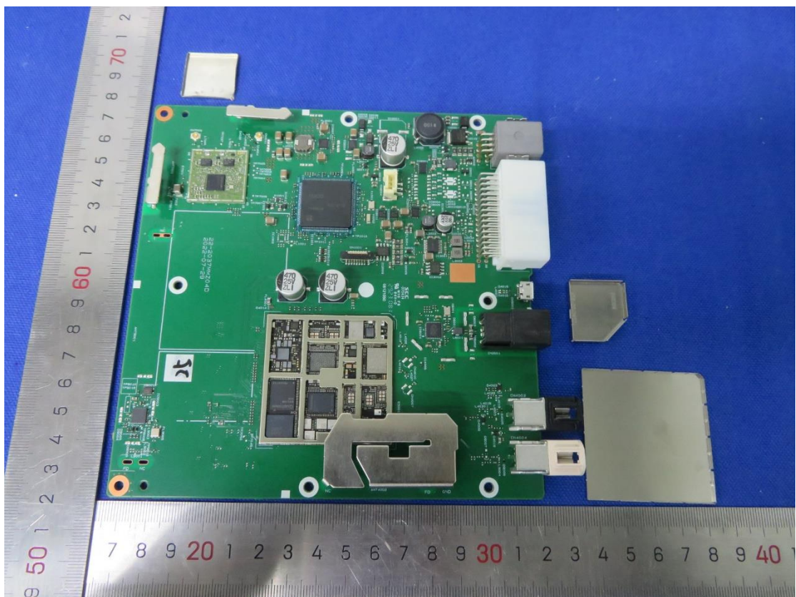
Internal View (shield-off)
