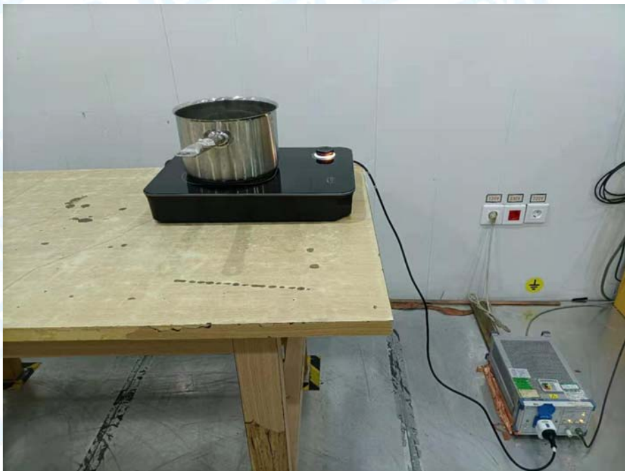
Photo of Setup for Conducted Emission
