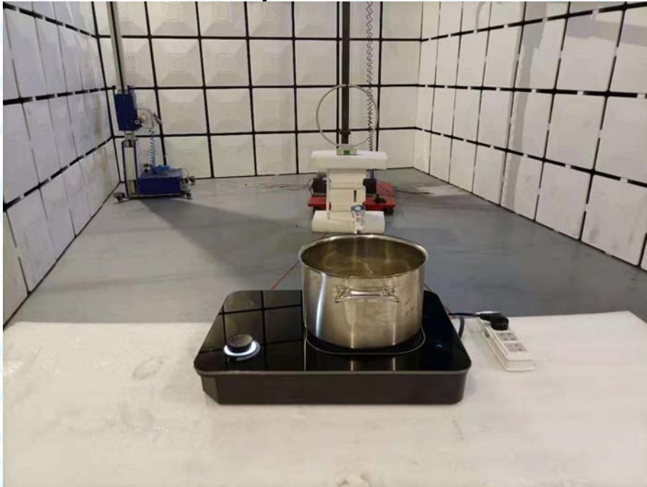
Photo of Setup for Radiated Emission
