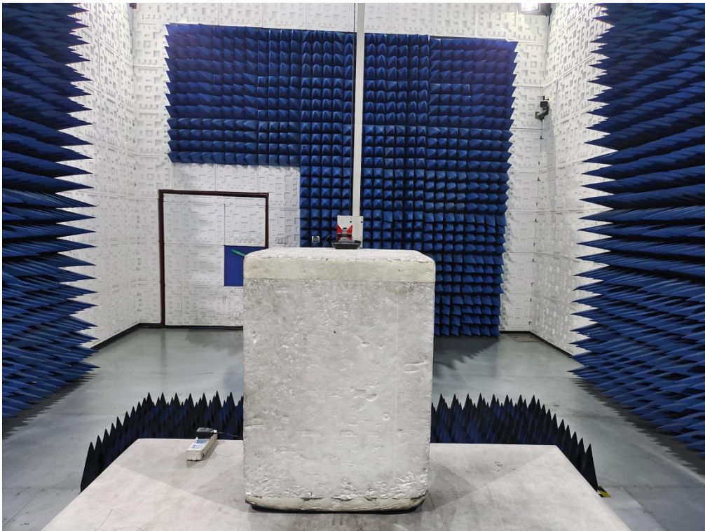
RADIATED EMISSION TEST SETUP ABOVE 1GHZ
