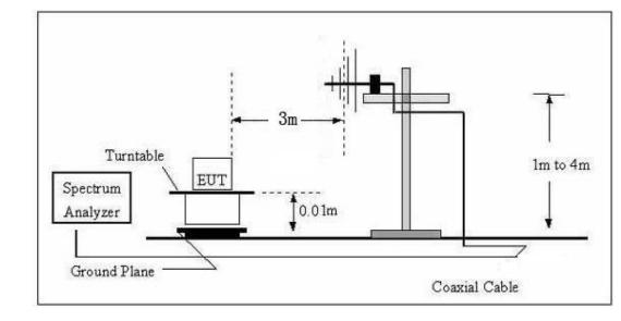
(C) For radiated emissions above 1000MHz
