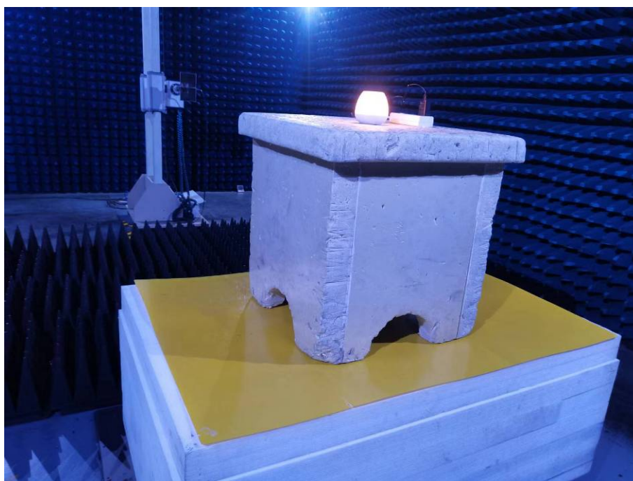
Photo of Radiated Emission Measurement (Above 1G)
