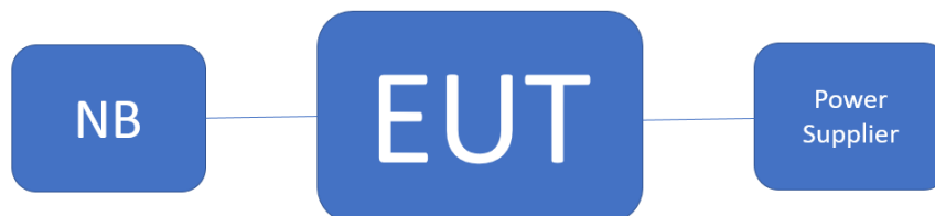
Fig. 2-1 Conducted (Antenna Port) & Radiated Emission Configuration & Emission from AC power line
