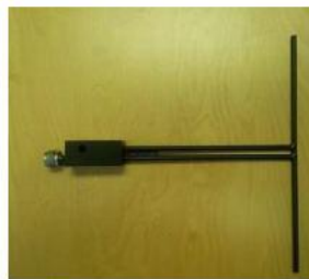
Figure 1 – MVG COMOSAR Validation Dipole
