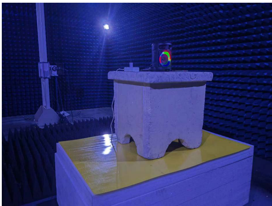
Photo of Radiated Emission Measurement Above 1GHz
