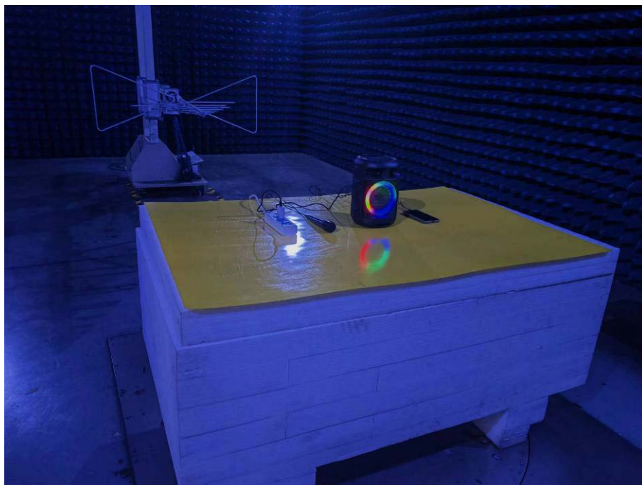
Photo of Radiated Emission Measurement Below 1GHz
