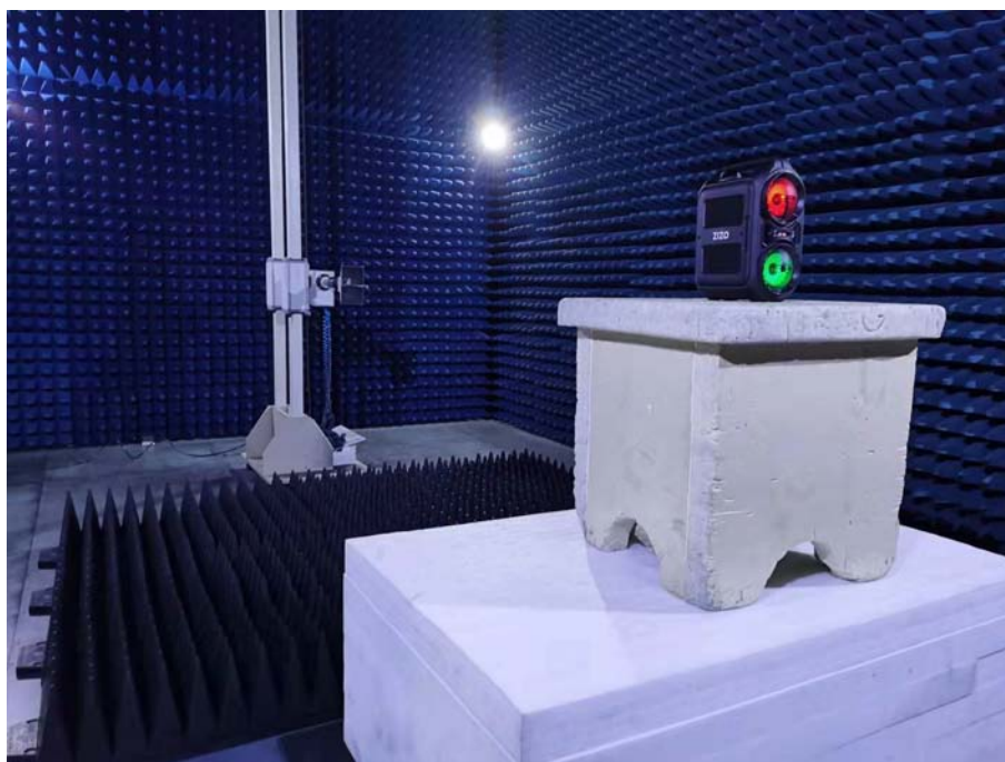
Photo of Radiated Emission Measurement Above 1GHz
