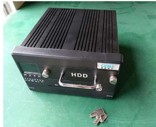
14、 Insert the assembled hard disk box into the device, tighten the fixing screws, and lock the hard disk lock. Note: If the hard disk box cannot be inserted, the hard disk box is reversed. Please adjust the front and back sides before inserting to prevent damage to the hard disk.
