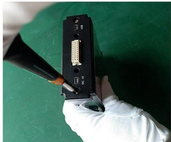
12、 After fixing the hard disk cover, fix it with screws
