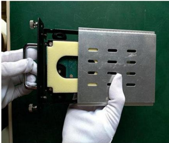
11、 As shown in the figure, put on the hard disk cover
