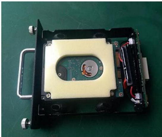
7. Fasten the fixed hard disk drive to the hard disk box
