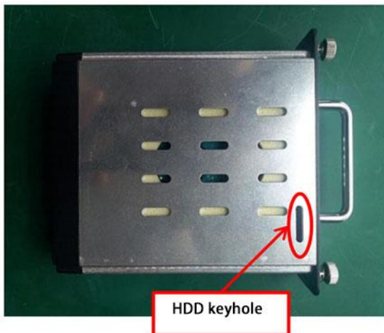
13、 The figure above shows the effect of the installed hard disk box. Note: The HDD keyhole should be close to the front panel of the hard disk box.
