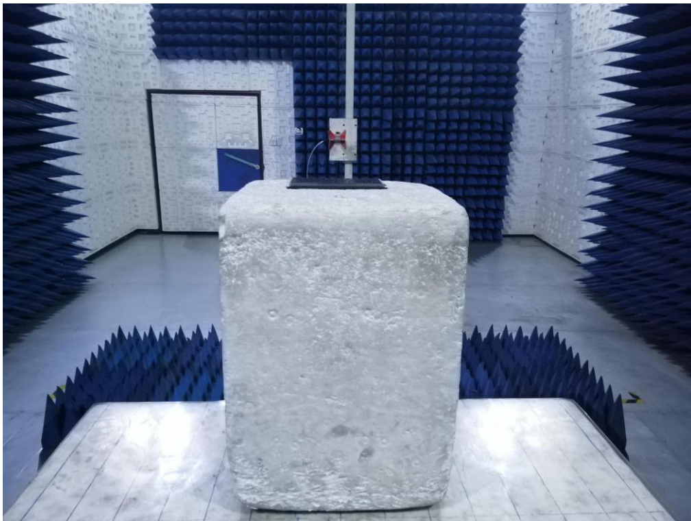
RADIATED EMISSION TEST SETUP ABOVE 1GHz
