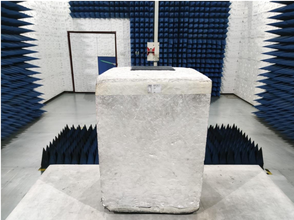
RADIATED EMISSION TEST SETUP ABOVE 1GHZ
