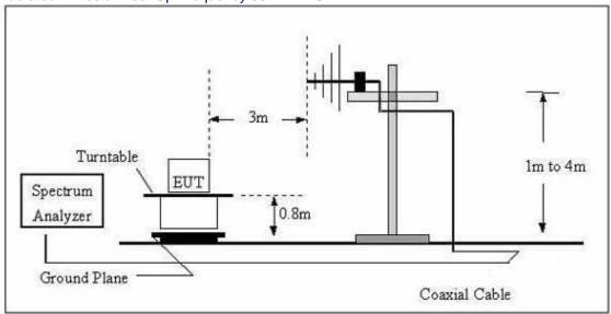
(C) Radiated Emission Test-Up Frequency Above 1GHz
