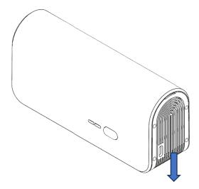
2. Gently pull the filter and take out the old filter, as shown in the figure
