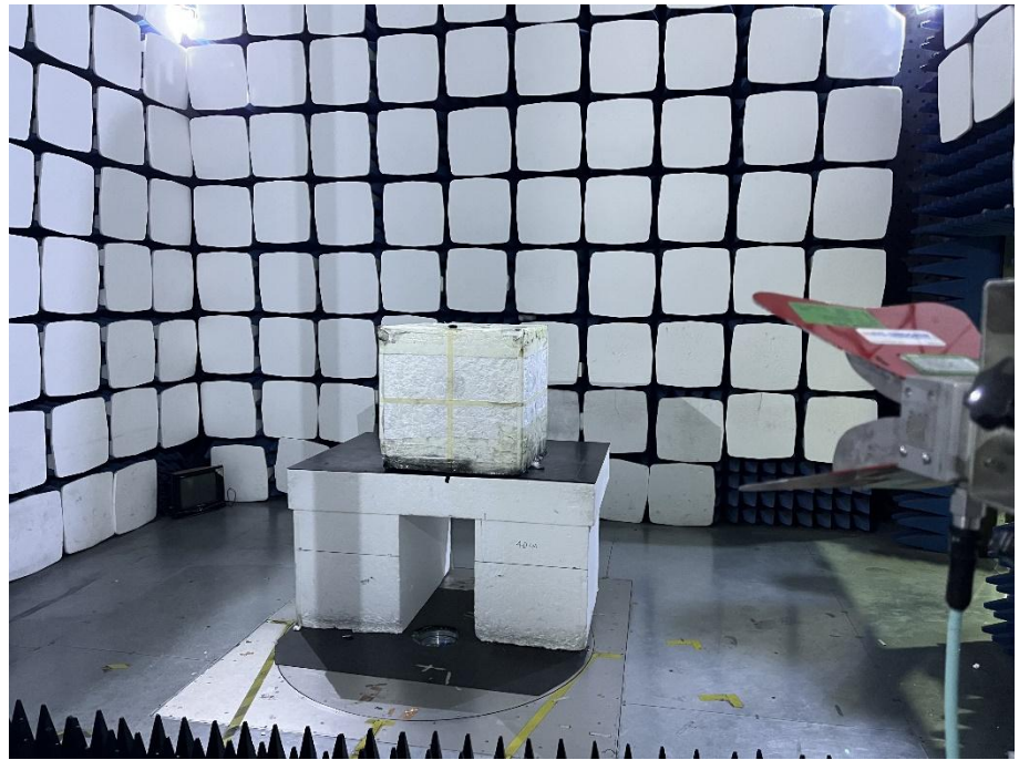
Radiation Emission Test Setup (1GHz to 18GHz)
