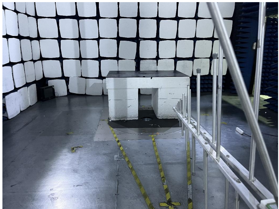
Radiation Emission Test Setup (30MHz to 1GHz)
