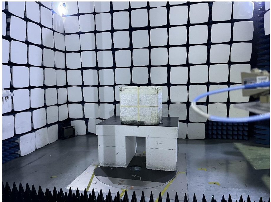
Radiation Emission Test Setup (Above 18GHz)
