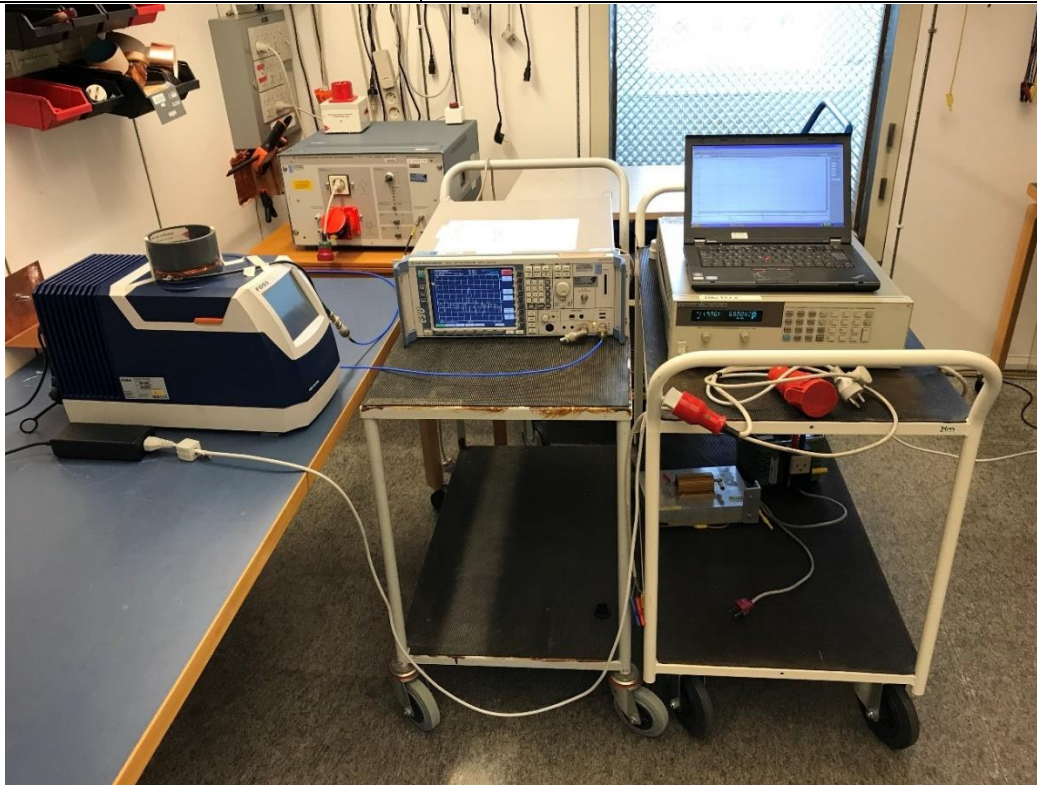
Photo 4.6.1 .....: Measurement of occupied bandwidth
