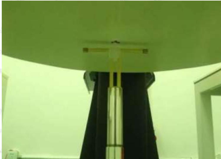
Photo of Dipole Setup
