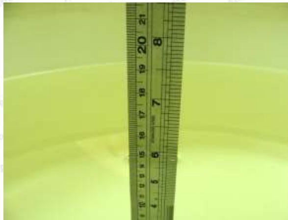
Photo of Liquid Height for Body SAR
