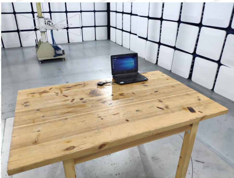
Photo of Radiation Emission Test
