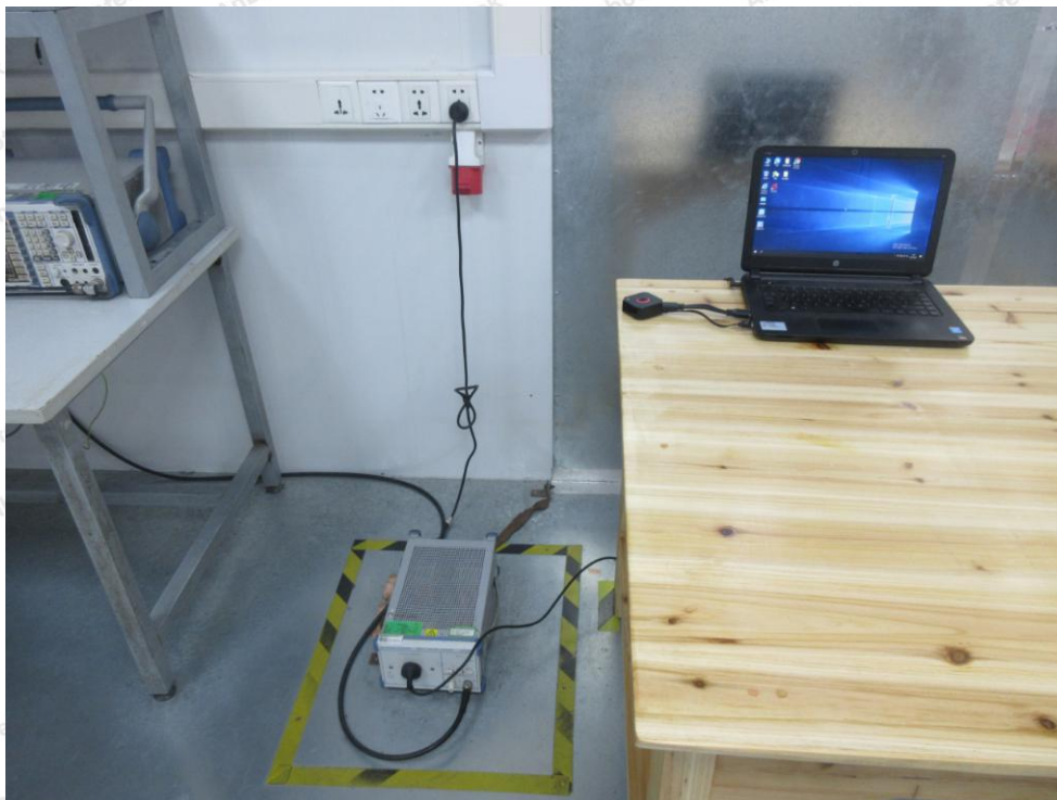
Photo of Power Line Conducted Emission Test
