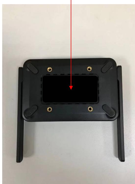
The label shown shall be permanently affixed at a conspicuous location on the device and be readily visible to the user at the time of purchase (Labeling requirements per 2.925)
