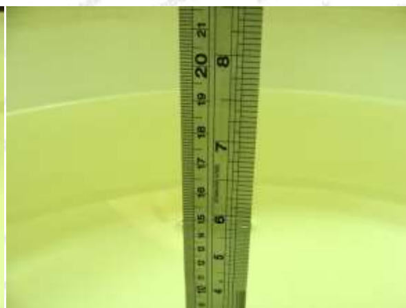
Photo of Liquid Height for Body SAR
