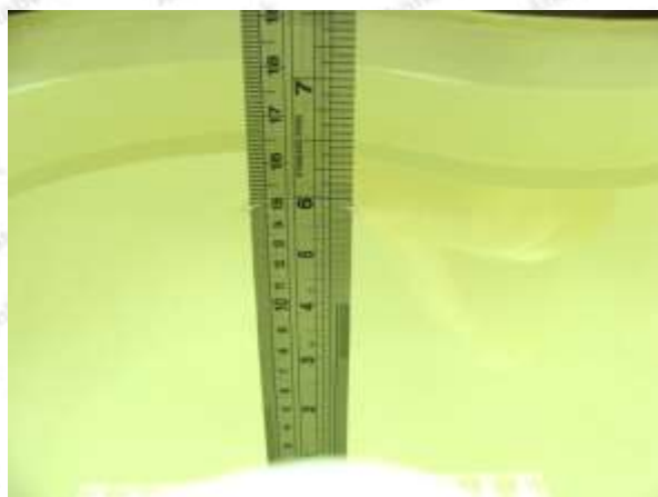
Photo of Liquid Height for Head SAR
