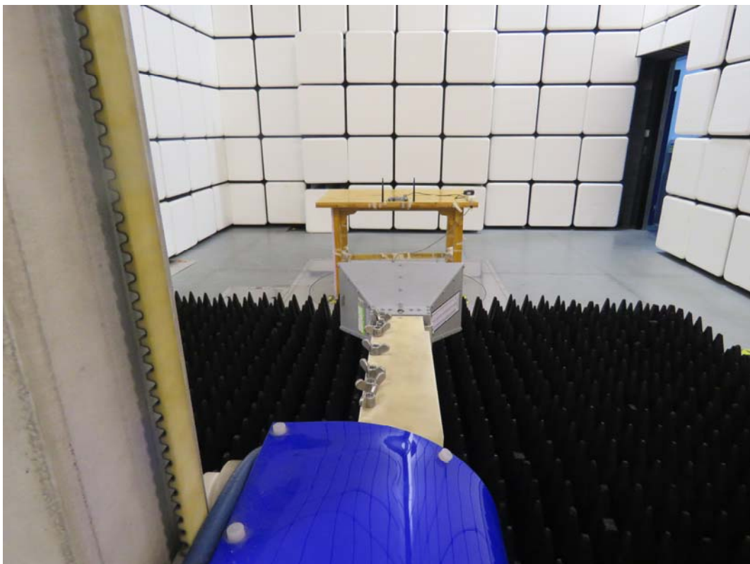
Picture 2: Radiated Spurious Emissions Test setup
