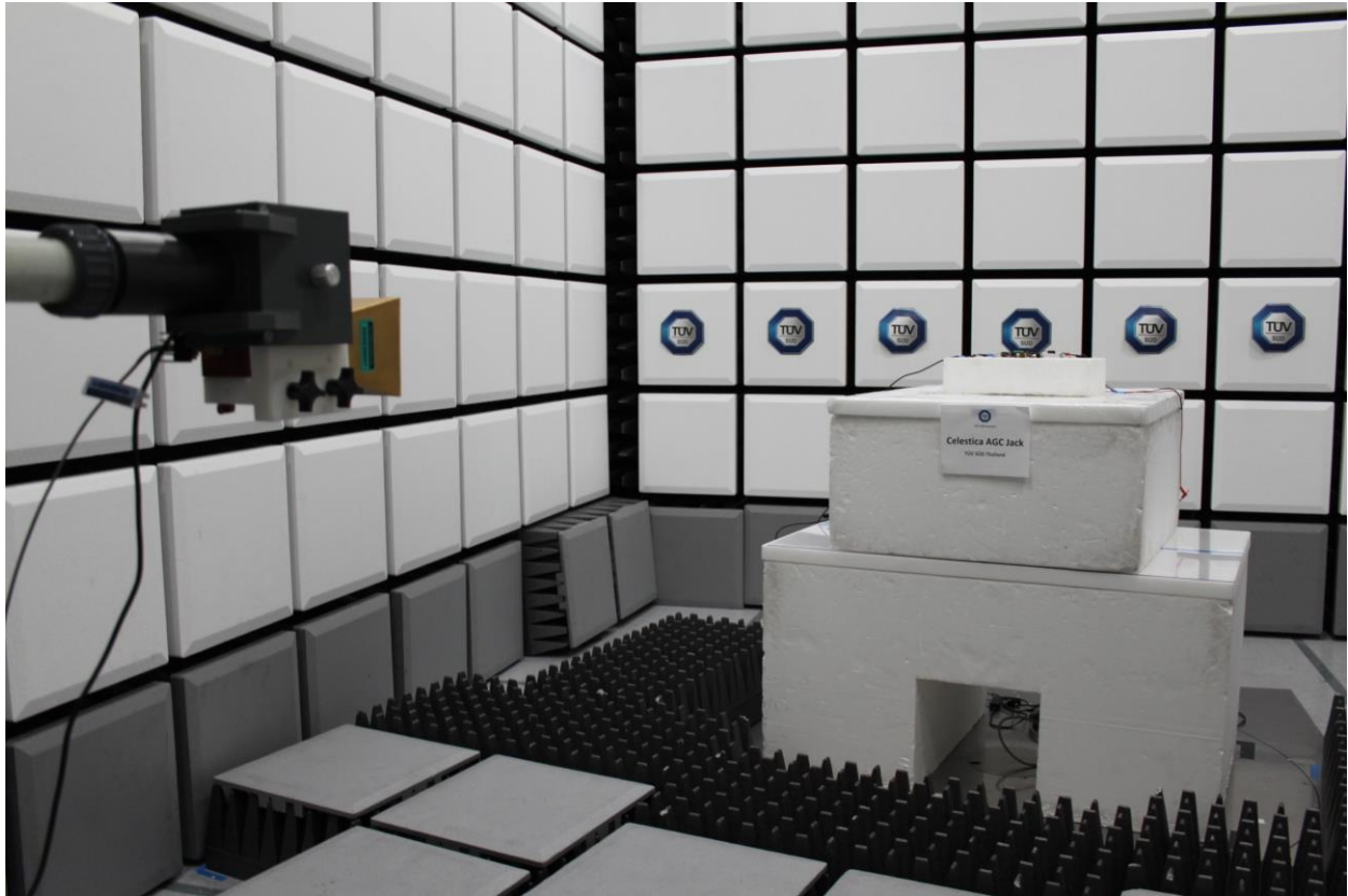
Radiated Emissions Test Setup (18GHz to 26GHz)
