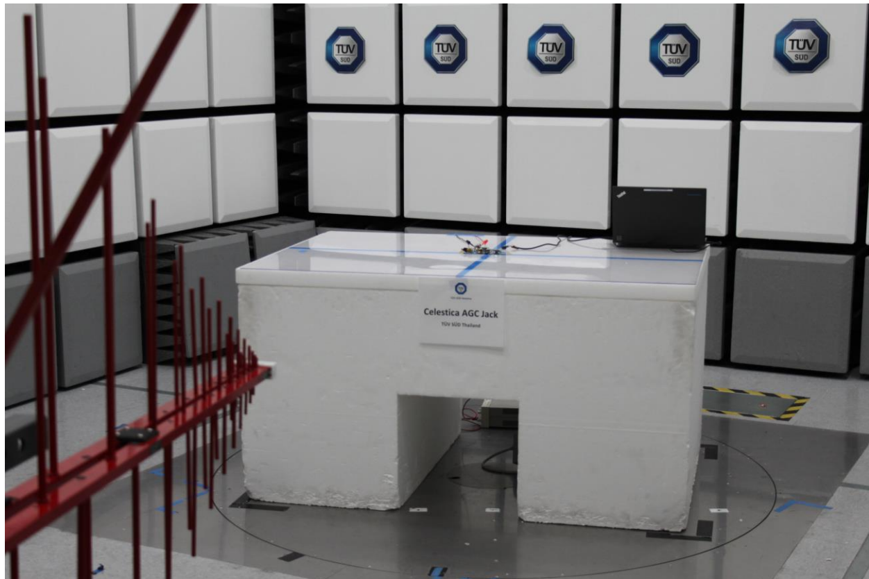
Radiated Emissions Test Setup (30MHz to 1GHz)
