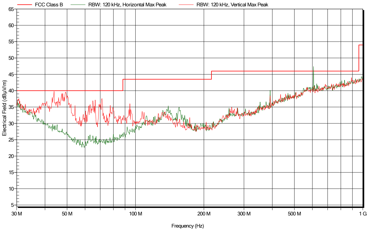
Figure 5.3.6.5: Electric field emissions Plot, 30MHz to 1GHz, operation on Channel 1 OFDM modulation- Peak detector scan
