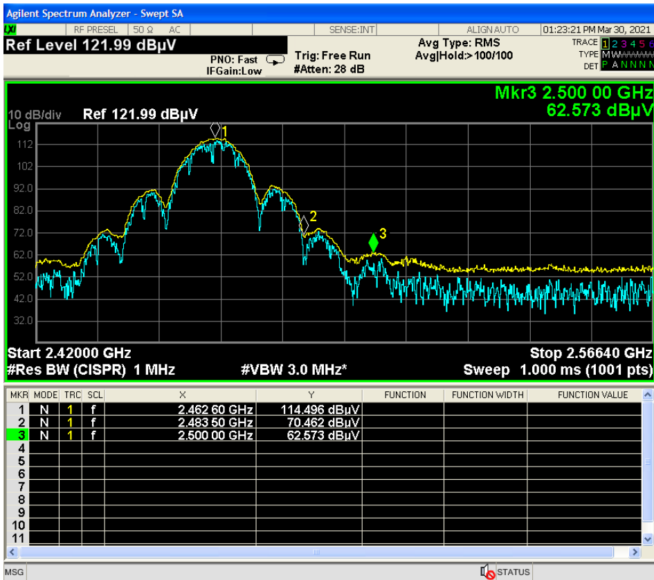
Band Edge Measurement – upper band edge – CCK modulation - vertical polarity
