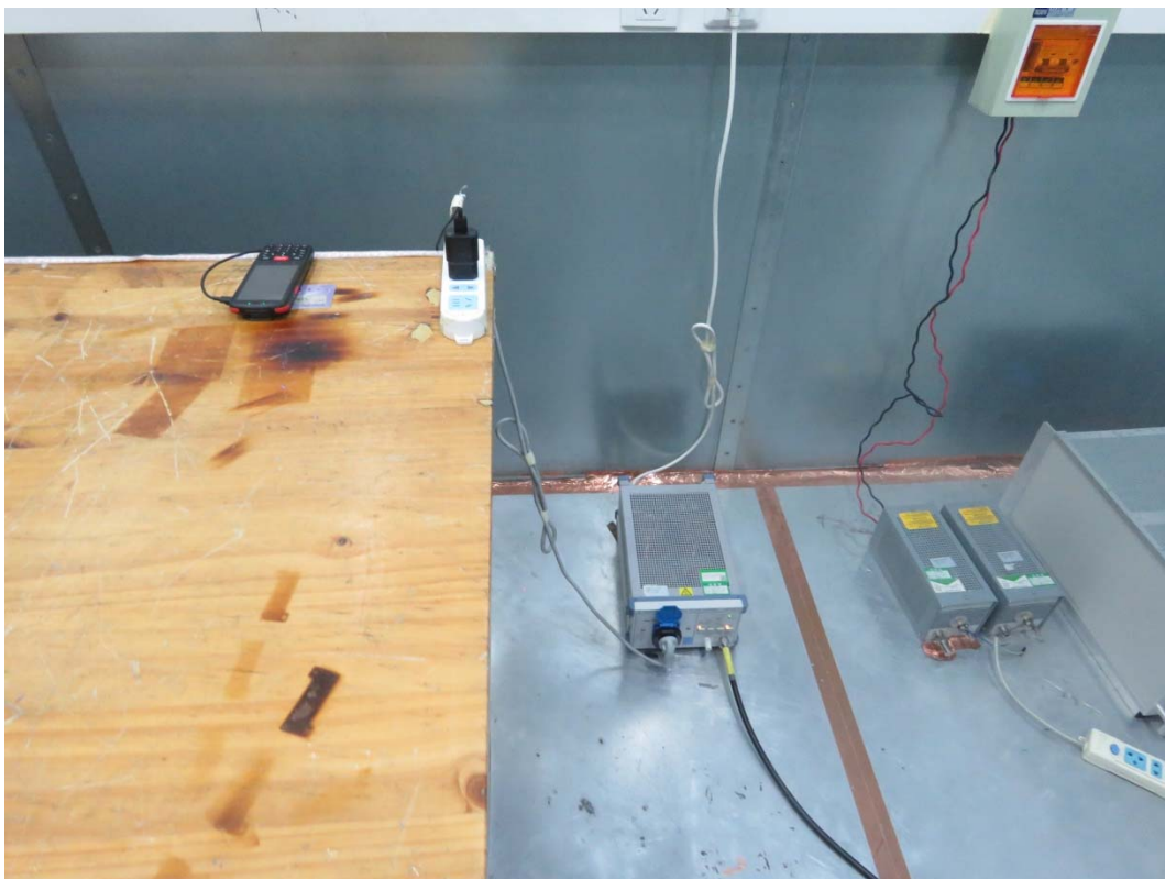
Picture 2 Conducted Emission Test Setup
