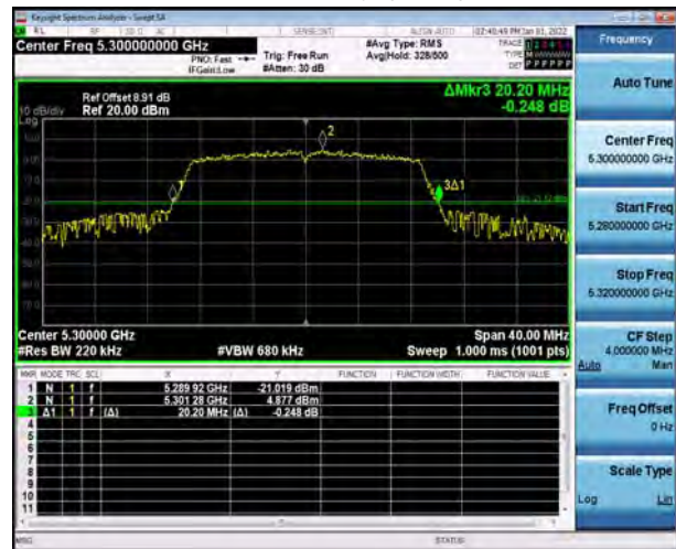
U-NII-2A, 802.11n HT20 Carrier frequency (MHz): 5300
