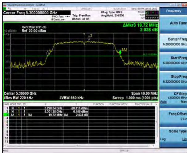
U-NII-2A, 802.11a Carrier frequency (MHz): 5300
