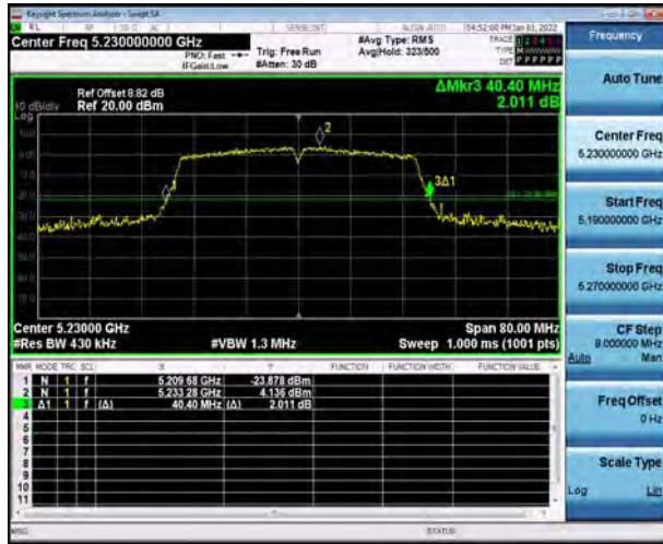
U-NII-2A, 802.11a Carrier frequency (MHz): 5260
