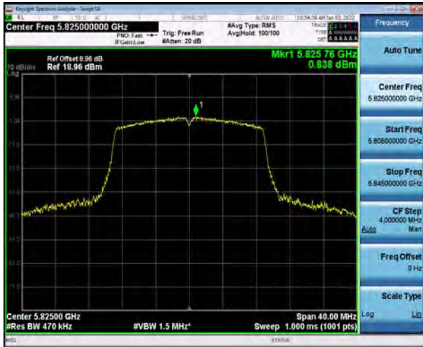
U-NII-3, 802.11ac VHT20, Channel No.: 149
