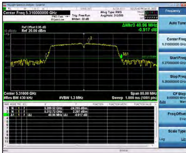
U-NII-2A, 802.11n HT40 Carrier frequency (MHz): 5310
