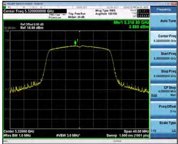
U-NII-2A, 802.11ac VHT20, Channel No.: 52
