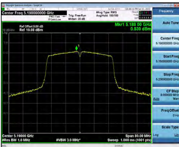
U-NII-1, 802.11ac VHT40, Channel No.: 38
