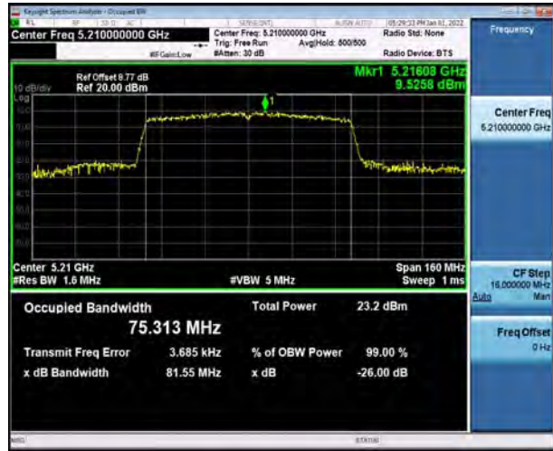
U-NII-2A, 802.11n HT20 Carrier frequency (MHz): 5260
