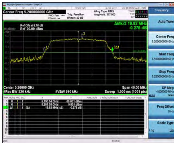
U-NII-1, 802.11a Carrier frequency (MHz):5240
