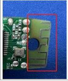
The antenna is PCB antenna. The best case gain of the antenna is -0.58 dBi.
