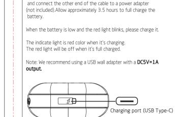
Plug the included USB type-C cable into the speaker's charging port,
