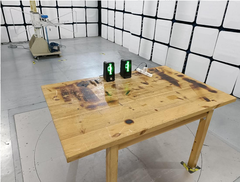
Photo of Radiation Emission Test
