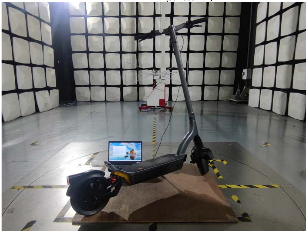
Radiated emission (30-1000MHz)
