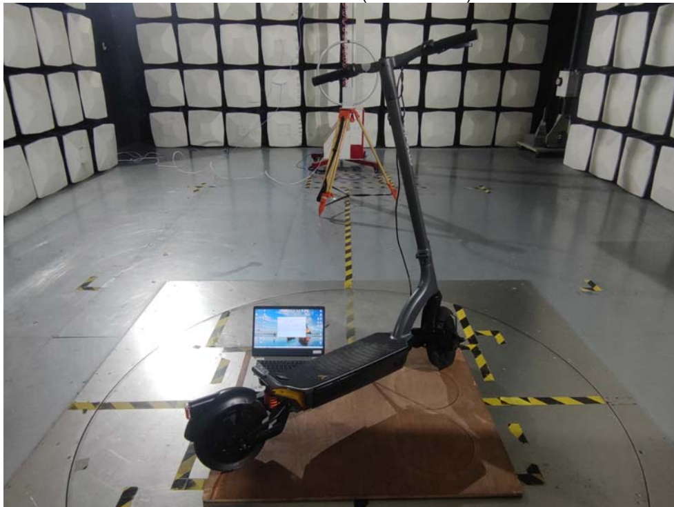
Test Photo Radiated emission (Below 30MHz)
