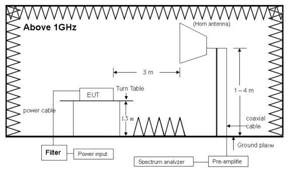
NOTE: The EUT system was put on a wooden table with 1.5m heights above a ground plane. For the actual test configuration, please refer to the photos of testing.
