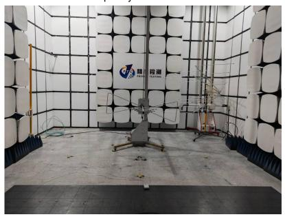
RADIATED EMISSION TEST
