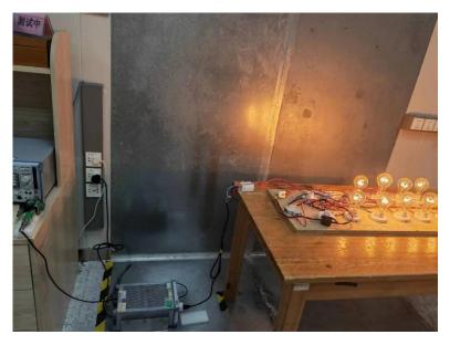
Radiated Emissions From 30MHz-1000MHz
