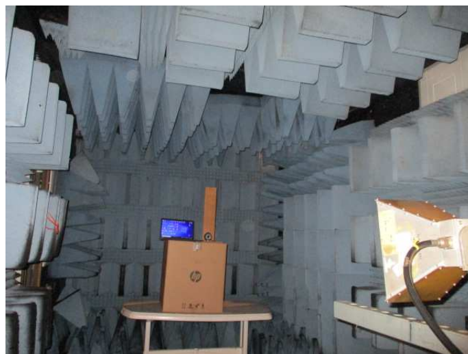
Figure 8. Radiated Emission Test, 1-18GHz
