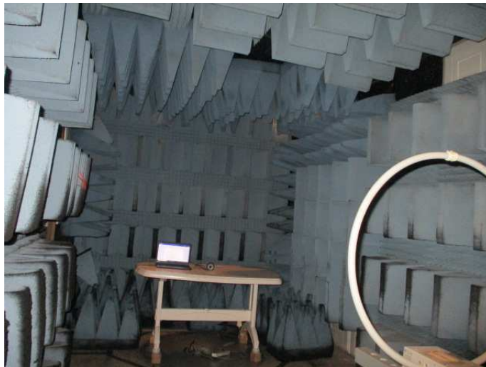
Figure 5. Radiated Emission Test, 0.009-30MHz
