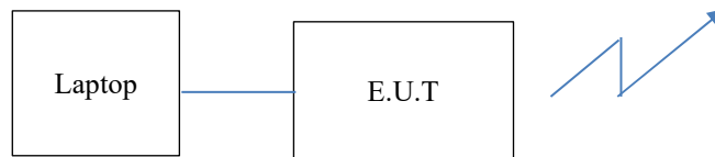
Figure 3. Configuration of Tested System - Radiated
