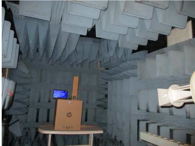
Figure 9. Radiated Emission Test, 18-25GHz
