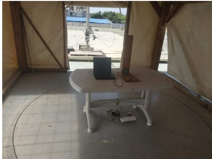
Figure 6. Radiated Emission Test, 30-200MHz
