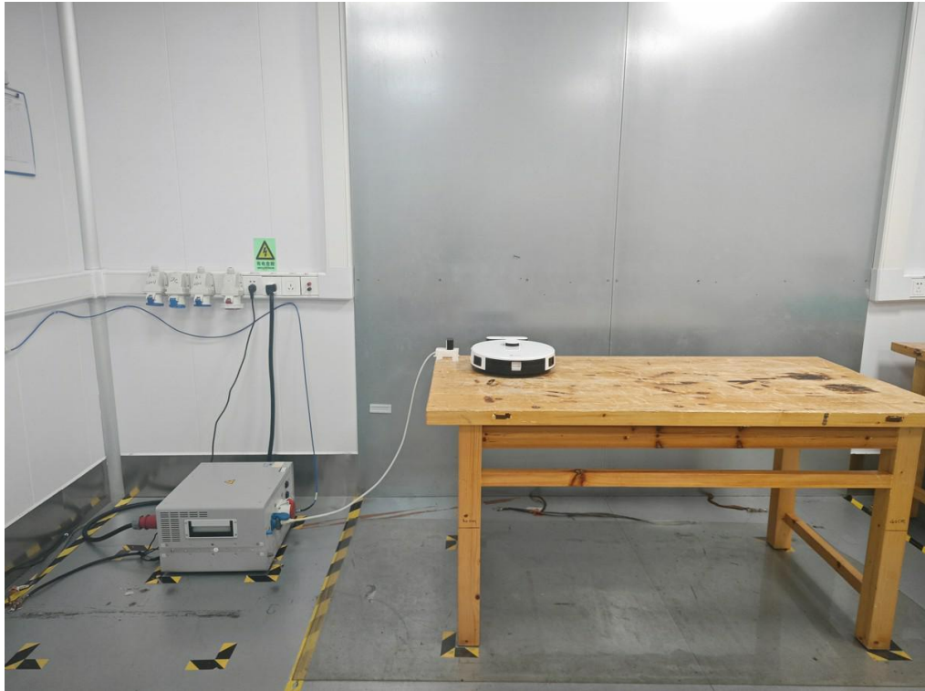
Conducted Emission at AC power line
