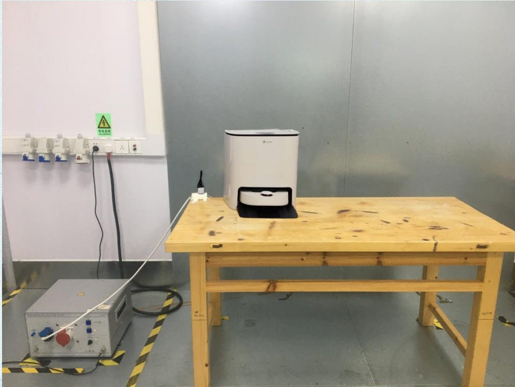
Conducted Emission at AC power line
