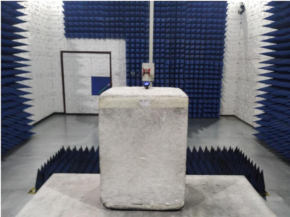
RADIATED EMISSION TEST SETUP ABOVE 1GHz
