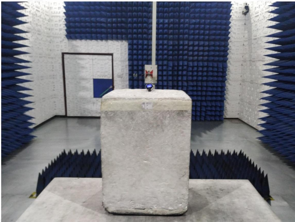
RADIATED EMISSION TEST SETUP ABOVE 1G
