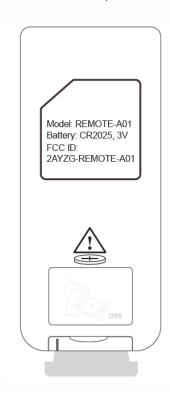
2. Open the battery compartment in the direction shown in the figure
