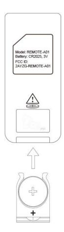
4. Insert the battery compartment in the correct direction
