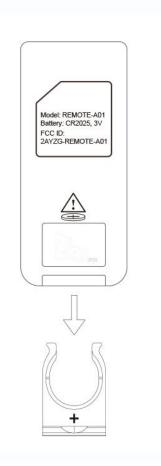
3. Facing the "+" and "-" pole marks of the battery compartment, put the 3v battery into the battery compartment
