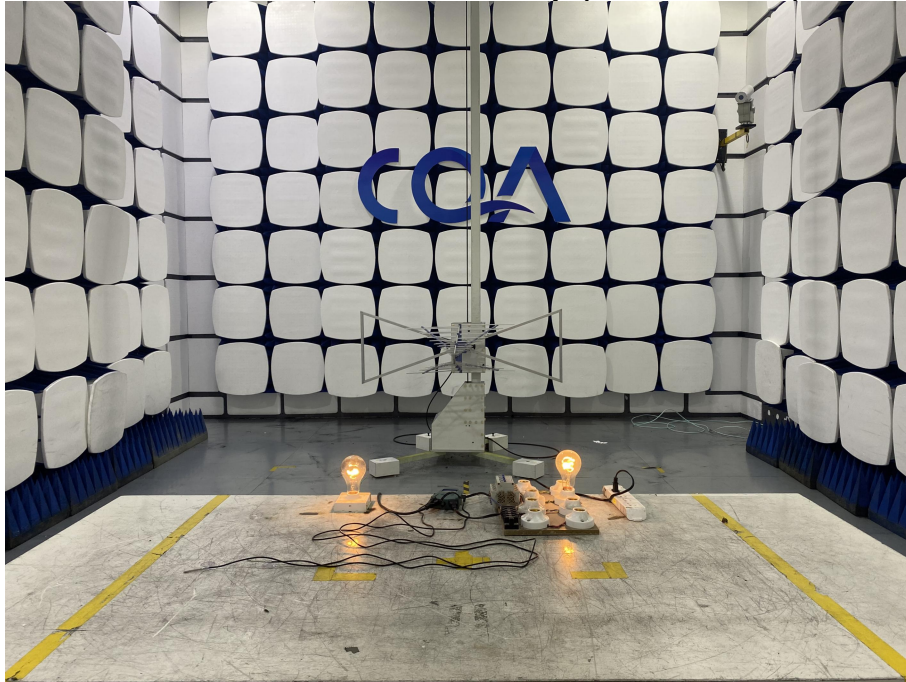
Radiated emission Test Setup (30MHz~1GHz)
