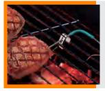
**NOTE:** When you detect the oven temperature or room temperature, you should fix the probe with a clamp to get stable measurement results.
